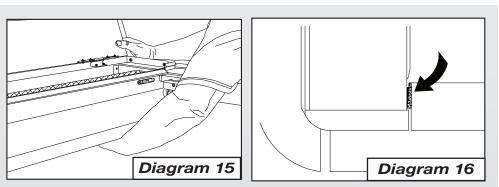
the inside surface of the tailgate. Make sure the Track End Cap Metal Blocks contact the Tailgate Extrusion End Caps (*Diagram 16*). Note that if the Tracks are not positioned as shown, the Latch Mechanism will not function correctly.
