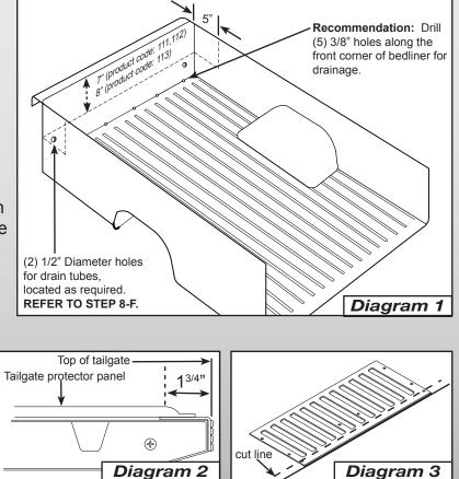
proceed to Step 2. If the plastic protector panel is above the line **remove** the panel and carefully make a straight cut to remove that portion of the panel **(Diagram 3)**. Replace the plastic protector panel.
